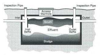
Effluent flows from the septic tank in the soil absorption system when displaced by incoming wastewater. A typical soil absorption system consists of gravel-filled trenches that are 18 to 30 inches deep. Perforated pipes run the length of these trenches. Effluent that is discharged from the septic tank flows through the perforated pipes, empties into the gravel trenches, and ultimately percolates through the underlying soil..
